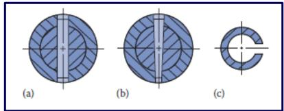
Some types of pins: (a) straight round pin, (b) tapered round pin, and (c) cross section of a split-tubular pin or so-called roll pin.
