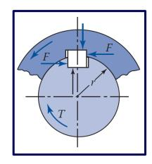
Shear and compressive or bearing stresses are calculated for the keys from force F, using a sufficiently large factor of safety. For steady loads, a factor of safety of 2 is commonly applied. On the other hand, for minor to high shock loads, a factor of safety of 2.5 - 4.5 should be used.
